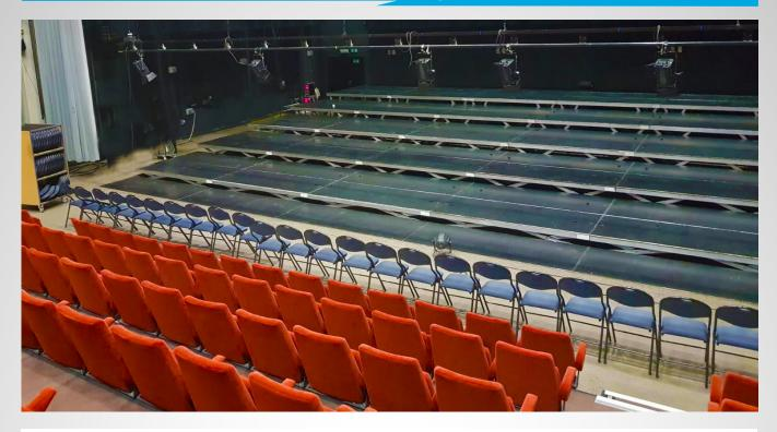
This platform system is ideal for stationary stage construction, because it is flush with the surrounding plane and can be simply lifted up when necessary.
