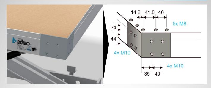
With BÜTEC compact corners made of zinc die-cast you have the possibility to mount accessories like railings and claddings fast and easy at the four corners of your BÜTEC platforms Servo Stage 1000 & 1500. By using threads M8 & M10 you can create strong and form-fit connections to the desired attachments.
