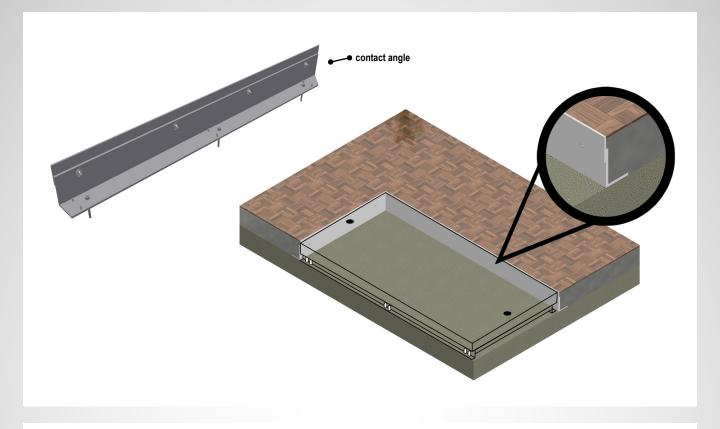
With BÜTEC edge angles made of aluminium you can easily realize a mounting pit for the BÜTEC Servo Stage 1000 and 1500. The edge bracket is fixed by screwing in the floor and a clean finish is made, which separates the pit from the surrounding floor area.
