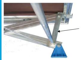
When constructing a 40 cm stage height, the scissor construction must always be secured with the support bracket. The articulated swivel feet compensate for slight unevenness or inclined positions.
