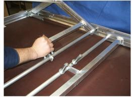
As a general rule, it is important to ensure that the platforms are mounted on a firm, level surface. The stability of the construction must be checked by the operator.
