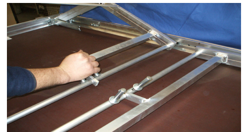
Scissor platform BÜTEC 100 here with screen print plate for outdoor use – water-proof laminated multi-layer plate, colour: dark Swivel feet with large contact areas provide a good load distribution, and a hinge allows compensation for sloping floors – without wobbling
