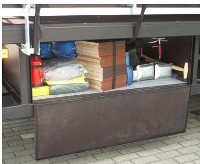
Lockable equipment compartment with basic safety equipment
