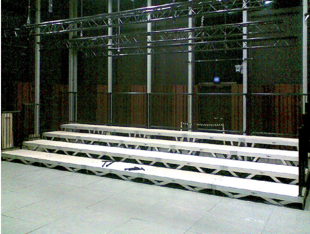
Application example: Tiering as stand – construction can also be used as stage.
